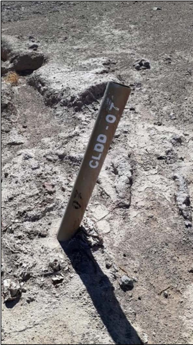
Figure 20: Drill Collar for Diamond Drill Hole CLDD-07 on the Cachinal Property
