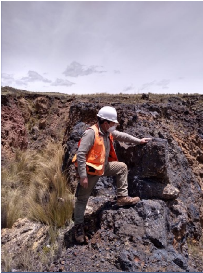
Massive manganese oxide replacing carbonates in old open pit
