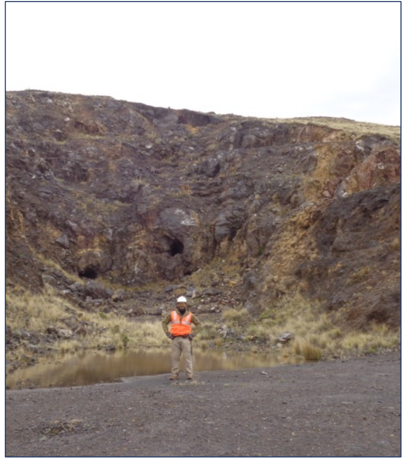
Old open pit & adits with MnOx replacing carbonates
