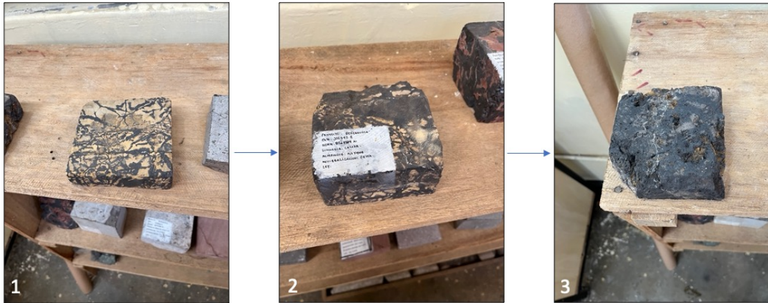
Progressive MnOx replacement of dolomite host rock along joints and fractures: (1) least intense to (3) complete replacement by massive MnOx
