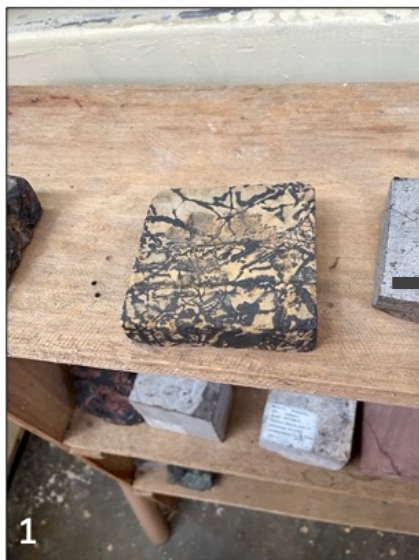
Progressive MnOx replacement of dolomite host rock along joints and fractures: (1) least intense to (3) complete replacement by massive MnOx
