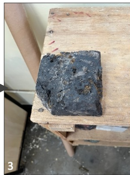
Progressive MnOx replacement of dolomite host rock along joints and fractures: (1) least intense to (3) complete replacement by massive MnOx
