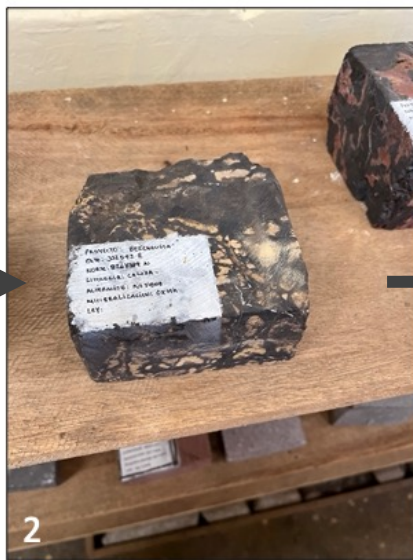
Progressive MnOx replacement of dolomite host rock along joints and fractures: (1) least intense to (3) complete replacement by massive MnOx
