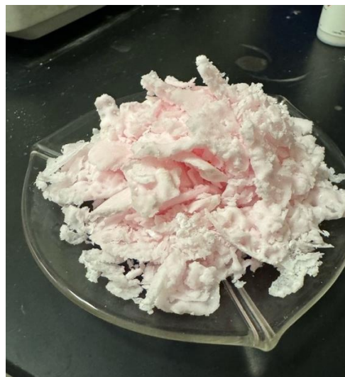
Figure 1. Battery grade crystallised \text{MnSO}_4 prepared by KCA from Berenguela composite sample.
