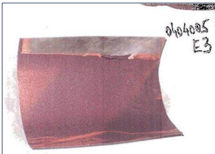
Figure 13-3: Photo of Cu plated to depletion (PRA, using EMEW Cells)
