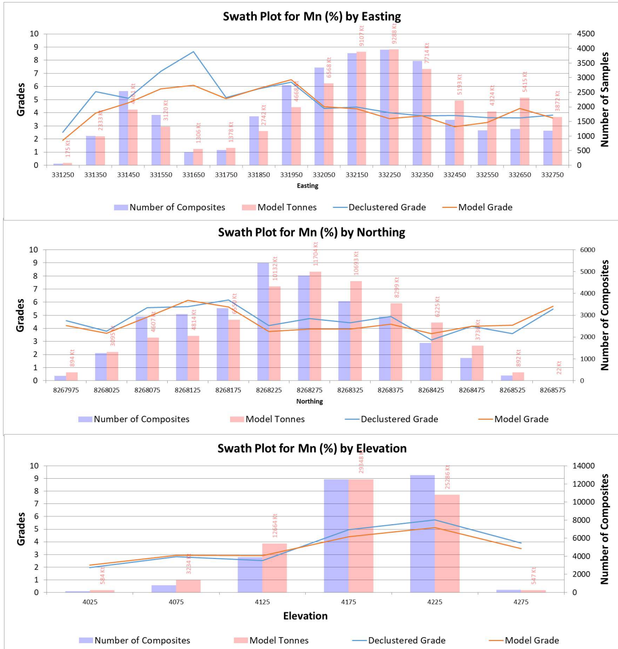
Figure 14-14: Swath plot for Mn (%) in Measured and Indicated blocks vs Composites
